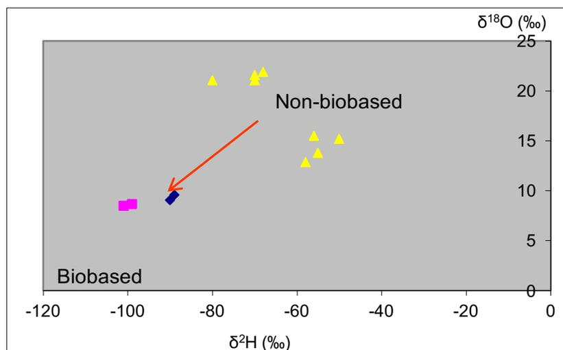
Figure 2: Representation of  $\delta^2\text{H}$  vs  $\delta^{18}\text{O}$  for PET plastic samples.
