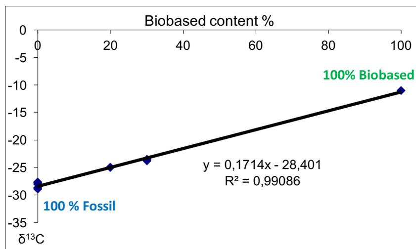
Figure 1: Representation of  $\delta^{13}\text{C}$  vs % biobased content on PET plastic samples
